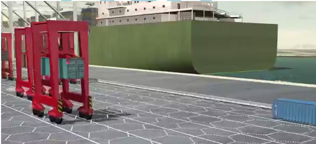
Automated Stacking Cranes (note GPS grids on the container yard) Source: G. Dombrowski
